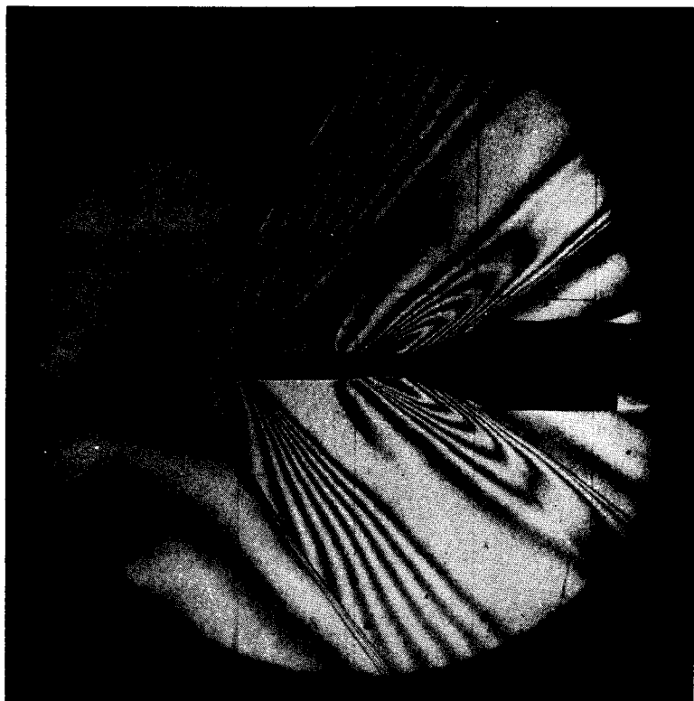
Fig. 48. Attached shock wave of a wedge. Mach number 1.45. The optical technique is the same as in Fig. 47. (Courtesy of Guggenheim Aeronautics Laboratory, California Institute of Technology.)
