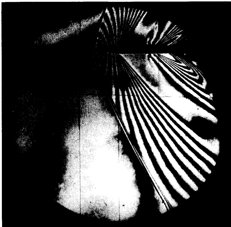
Fig. 47. Detached shock wave of a wedge. Mach number 1.32. The details of the flow field are made visible by the use of an interferometer . Light and dark fringes indicate surfaces of equal air density. (Courtesy of Guggenheim Aeronautics Laboratory, California Institute of Technology.)
